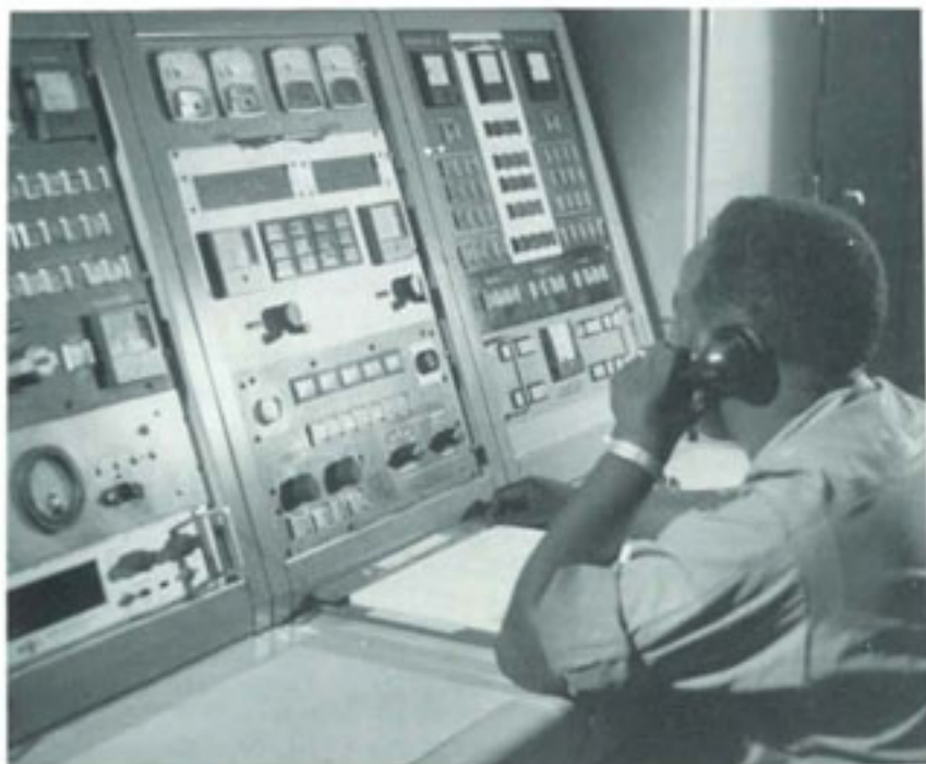
CONSOLE OPERATOR AT SAIGON SATELLITE TERMINAL. Soldier monitors satellite traffic and selects satellite to be used.
