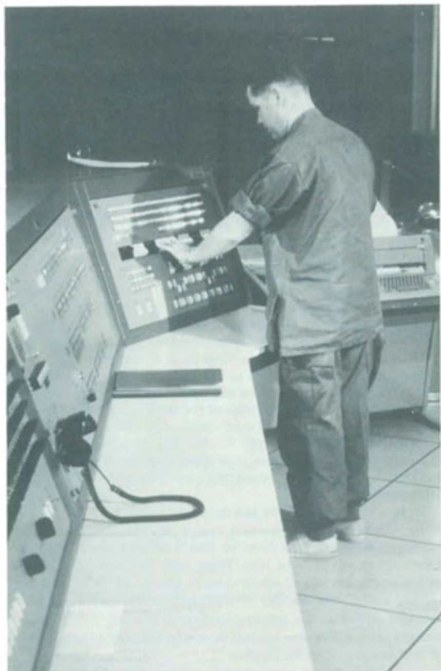
CHECKING A CONSOLE AT PHU LAM AUTOMATIC MESSAGE SWITCHING CENTER. White rubber-soled shoes were required in dust-free, temperature-controlled building necessary for equipment.
